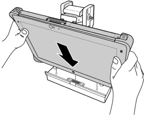
2. Secure the R11L tablet PC by pulling the latch forward until a "click" is heard and the latch is fully engaged.
