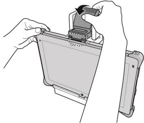
3. Fully push the latch bar into position to ensure the latch is tightly secured.
