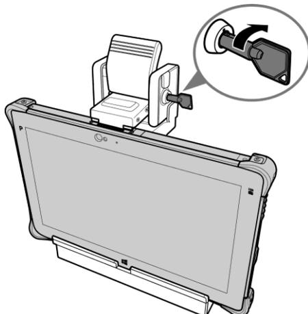
2. While supporting the R11L tablet PC with one hand, push the latch backward until it fully disengages.
